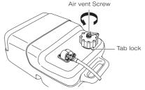
② For the 30, 40 and 50 models, insert the fuel connector into the connector in the engine side.
