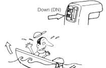
Improper Trim Angle (bow dips into the water)
