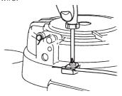
3 Remove the upper portion of the starter lock wire.
