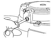
2 Loosen the screw for starter lock wire.
