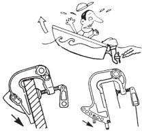
Set the thrast rod lower Remark) Thrust rod is for MF and EF, and preset knob is for EP.
