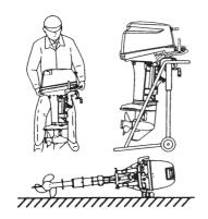
Keep the outboard motor in a vertical position when carrying.
