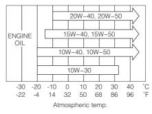
You can also use NMMA FC-W certified 4-stroke outboard oil below. 10W-30: is recommended for use in all temperature.
