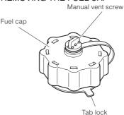
IMPORTANT: Contents may be under pressure. Rotate the fuel cap 1/4 turn to relieve pressure before opening.
