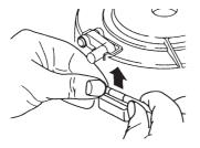
4 Remove the lower portion of the starter lock wire.
