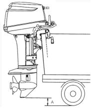
A:Ground clearance should be provided sufficiently.
