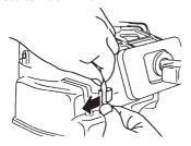
(5) Remove the bolts (3cps), and remove the recoil starter assembly.
