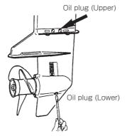
(2) Insert the oil tube nozzle into the lower oil plug hole, and fill with gear oil by squeezing the oil tube
