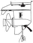
(2) Insert the oil tube nozzle into the lower oil plug hole, and fill with gear oil by squeezing the oil tube
