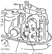
High pressure fuel filter Fuel filter
