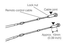
② Fitting of Remote Control Cable to Engine
