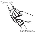
4) Be sure to install the stop switch lock to the stop switch.
