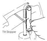
② Return to normal running position Move (UP) lock lever to "Free" position. Outboard motor moves down to thrust rod. Move (DOWN) lock lever to "Lock"
