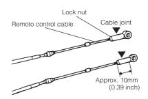
2 Fitting of Remote Control Cable to Engine
