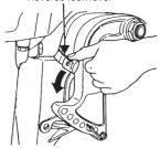
② Return to normal running position: Put the reverse lock lever in the tilt down position, slightly lift up the outboard motor, and then put it down.
