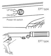
It is possible to tilt up or down in spite of main switch "ON" or "OFF".
