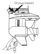
3 Install the upper oil plug, and then remove oil tube nozzle and install the lower oil plug.
