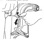
② Return to normal running position: Put the reverse lock lever in the tilt down position, slightly lift up the outboard motor, and then put it down. Reverse lock lever
