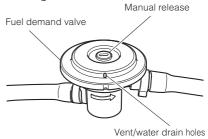
Fuel demand valve - installed in the fuel hose between the fuel tank and primer bulb.
