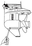
2) Insert the oil tube nozzle into the lower oil plug hole, and fill with gear oil by squeezing the oil tube until oil flows out of the upper plug hole.
