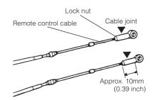
② Fitting of Remote Control Cable to Engine.
